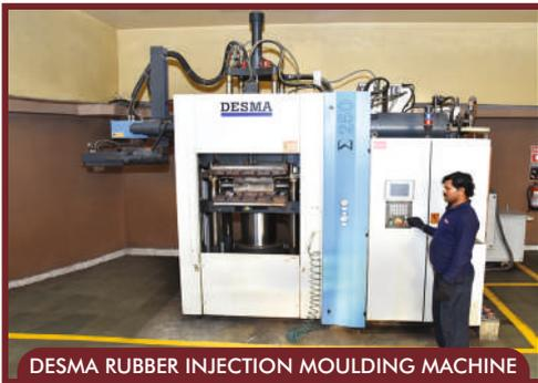
DESMA RUBBER INJECTION MOULDING MACHINE
