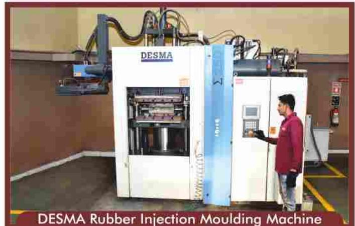
DESMA Rubber Injection Moulding Machine
