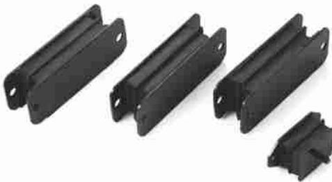
The sandwich mountings are available in 2 sizes. Can be fitted under direct compression or at different inclinations to suit diverse applications. These can be used for small engines with mobile applications, hoppers, carriage construction etc.
