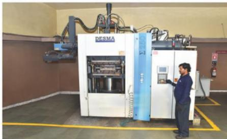
DESMA Rubber Injection Moulding Machine
