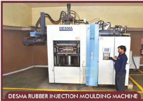
DESMA RUBBER INJECTION MOULDING MACHINE
